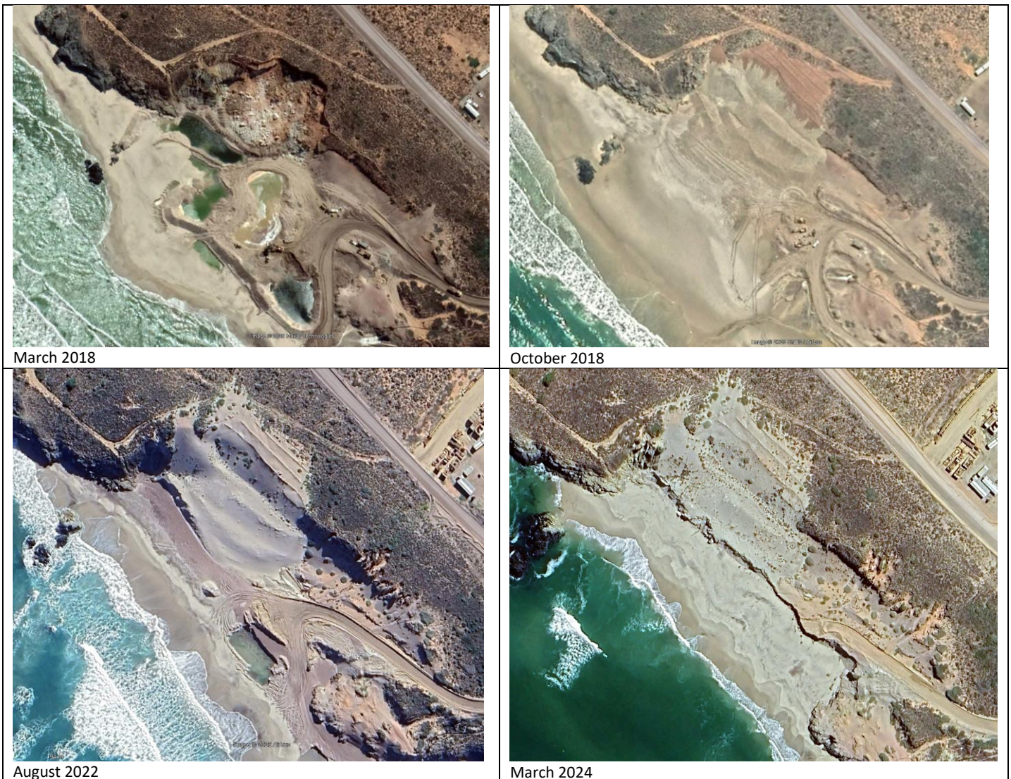
Photos 1: Shows the extensive remodelling of the slumped NW corner of the operation largely related to the actions of MSR while the SE corner of the photos show the final phase of THG mining operations on the site at the time of photography.
